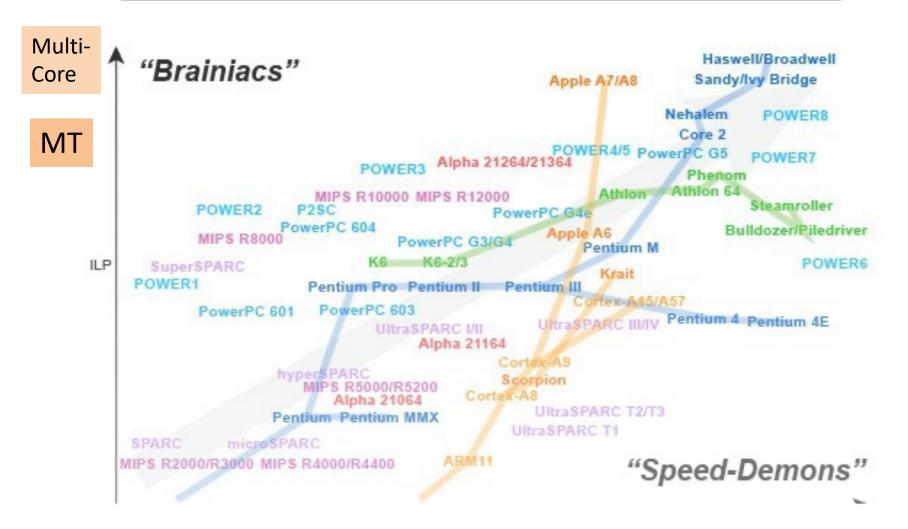
image: CPU Architecture War: Clock Speed v.s. Instruction-Level Parallelism [
