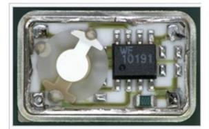
Inside a modern DIP package quartz crystal oscillator module. It includes a ceramic PCB base, oscillator, divider chip (/8), bypass capacitor, and an AT cut crystal.
