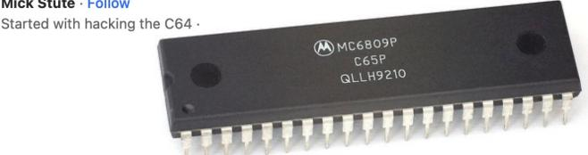
The 6809 was the first microprocessor that a programmer could write completely position independent fully reentrent code without using coding tricks — in other words, the chip fully supported it making designing and writing such a program "easy". This is because the stack registers had some advanced addressing modes and and the addition of the user stack pointer "U" and it provided addressing relative to the PC.
