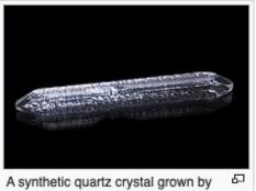
A synthetic quartz crystal grown by the hydrothermal synthesis, about 19 cm long and weighing about 127 g
