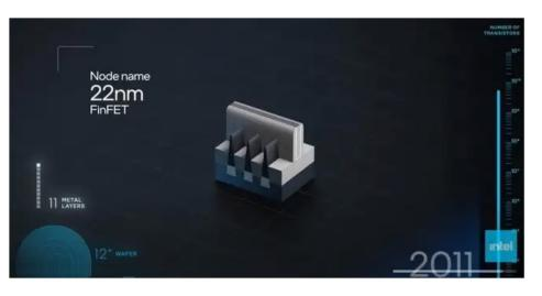
Intel amazed the industry with its aggressive adoption of a new transistor topology at the 22nm process node – the FinFET (also known as the "tri-gate FET").
