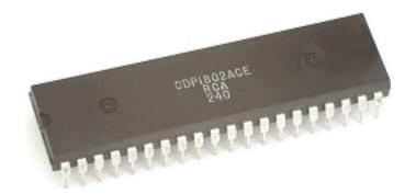
So it could be run, for example, at a clock speed of 1 Hz. Since most instructions took 16 clock cycles, it would take 16 seconds to execute an instruction. But it could be run much slower, and still execute (0.1 Hz, 0.01 Hz etc).
