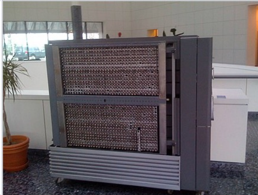
IBM 701 processor frame, showing 1071 of the vacuum tubes
