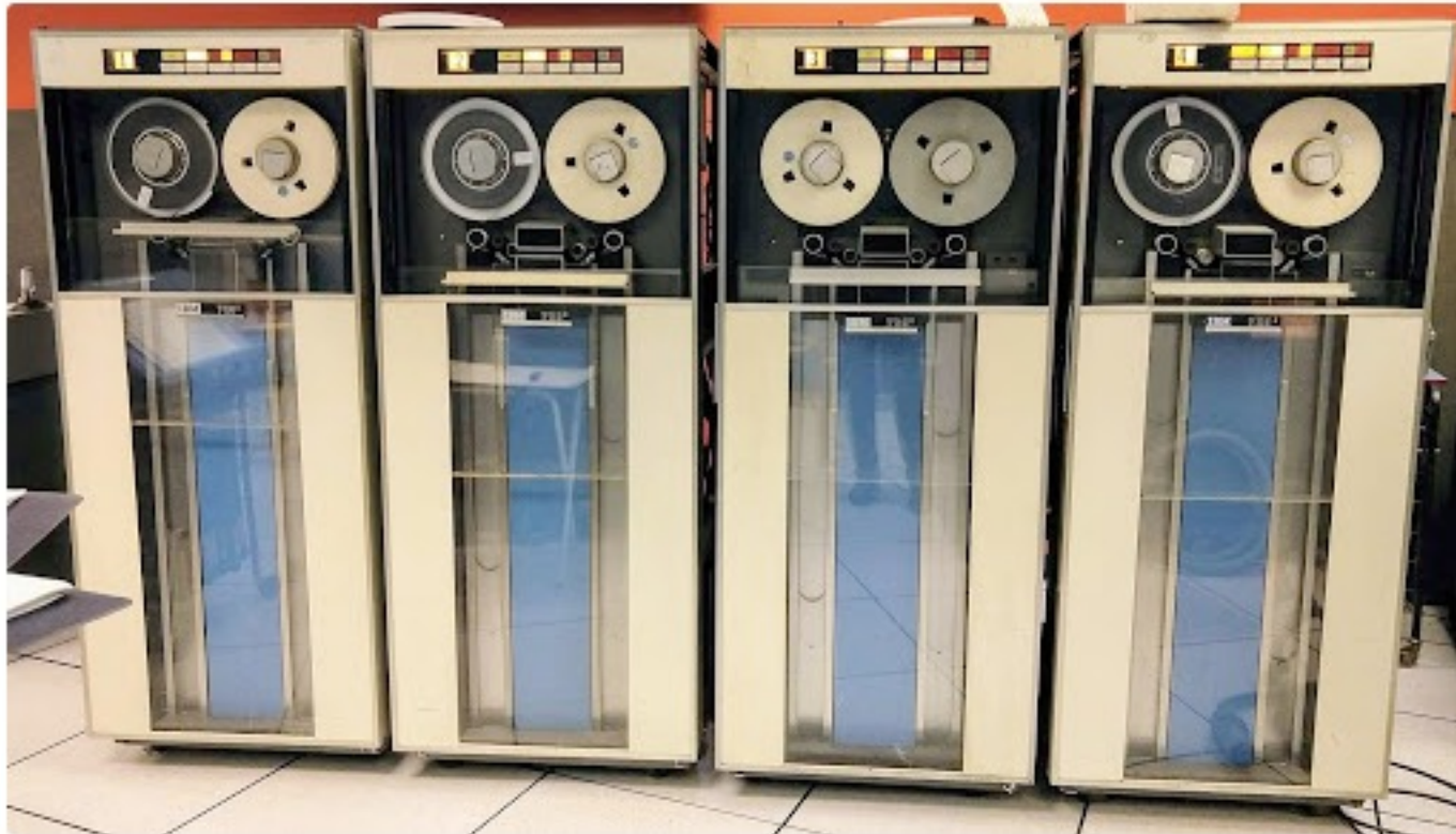
IBM 729 Tape Drives — with vacuum tape loop buffering
