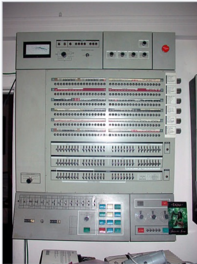
System/360 Model 65 operator's console, with register value lamps and toggle switches (middle of picture) and "emergency pull" switch (upper right)
